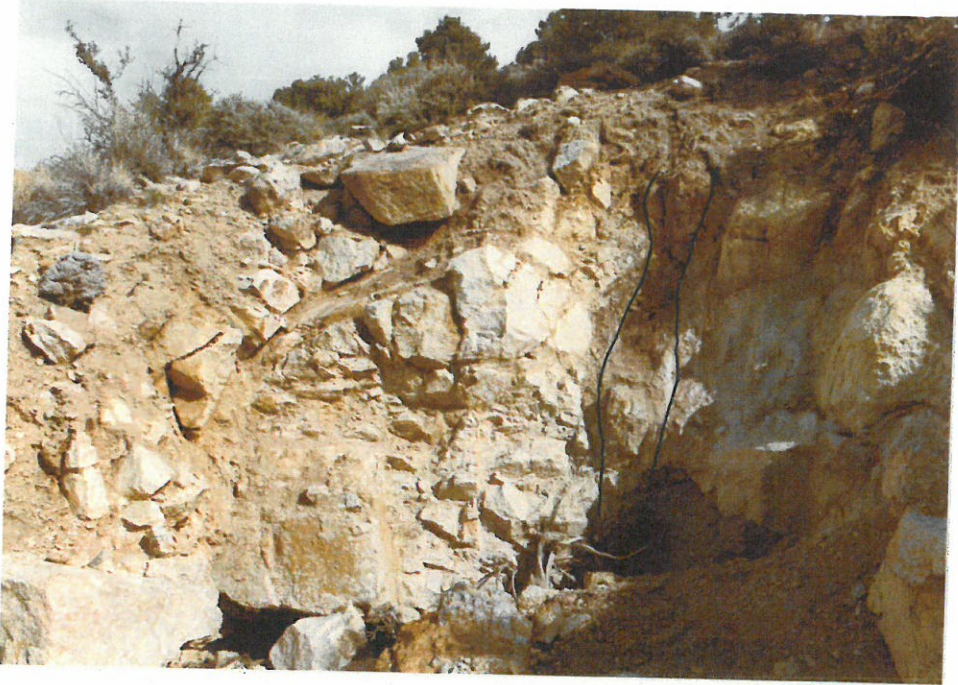
Plate 4. Adit opening on Sunshine Annex claim showing near vertical quartz vein ten inches (25 cm) thick surrounded by pale green altered Sylvania quartz monzonite.
