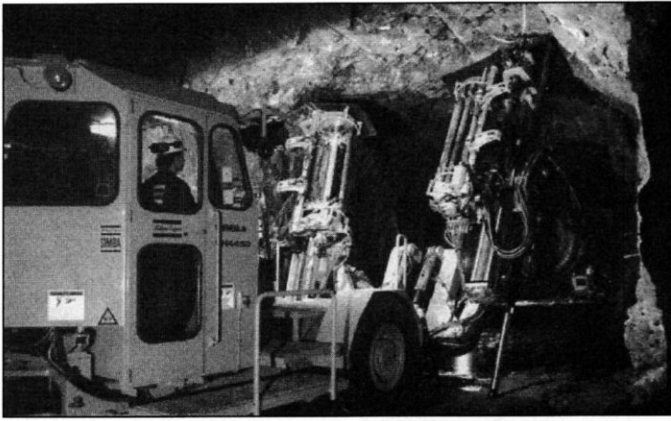
FIGURE 1.23 Twin boom rig for fan drilling, with operator's cabin, tube handling, and drill automatics, Kiruna, Sweden
