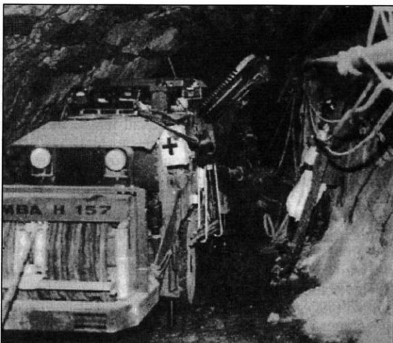
FIGURE 1.7 Mini-rig for longhole drilling, Stillwater platinum mine, Montana, USA
