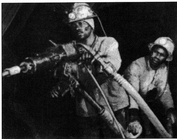
FIGURE 1.21 Drilling the reef with hand-held rock drill, East Rand Properties, South Africa
